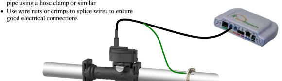
Note: If the Grundfos VFS sensor is not properly grounded to the Apollo and the pipe, it may not provide accurate flow measurements
